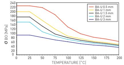
σ<sub>BO</sub> diagram represents σ<sub>BO</sub> values for different gasket material thicknesses. These values indicate the maximum in-service compressive pressures which can be applied on the gasket area involved without destructing or damaging the gasket material.
